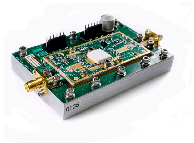
FIGURE 2: Pin and Socket Pallet IGNP1214L250 inserted into its test fixture
