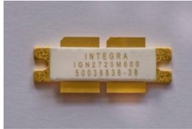
Fig. 3 – Picture of 1kW pulsed transistor
