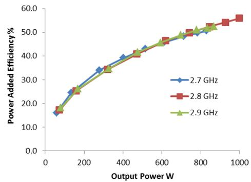
Fig. 5 – Power Added Efficiency vs output power.
