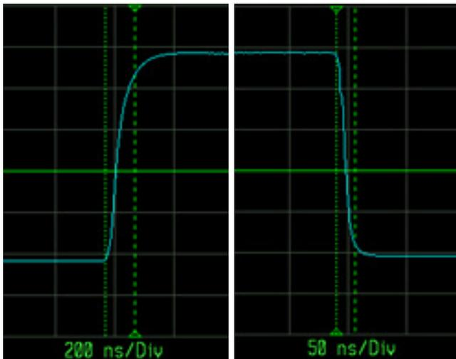
FIGURE 3: RF output Waveform with Gate Pulsing
