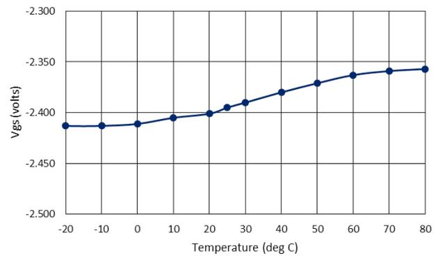
FIGURE 8:  $V_{GS}$  vs. Temperature for Constant  $I_{DQ}$ .
